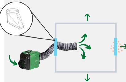
To create a positive pressure: Locate the Raptor outside the internal space. Fix the 3m x 250mm flexible ducting to the unit. Feed the ducting in through a window; the fishtail can be used to reduce the opening. When switched on, the Raptor will force clean air into the room and force contaminated air out through windows and vents. The high airflow will maintain a positive pressure environment.
