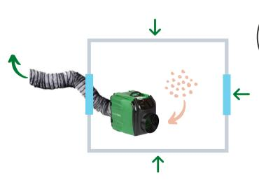
To create a negative pressure: Locate the Raptor within the internal space. Fix the 3m x 250mm flexible ducting to the unit. Feed the ducting out through a window; the fishtail can be used to reduce the window opening. When switched on, the Raptor will extract the contaminated air from inside the room and vent it outside the room. The high airflow will maintain a negative pressure environment.
